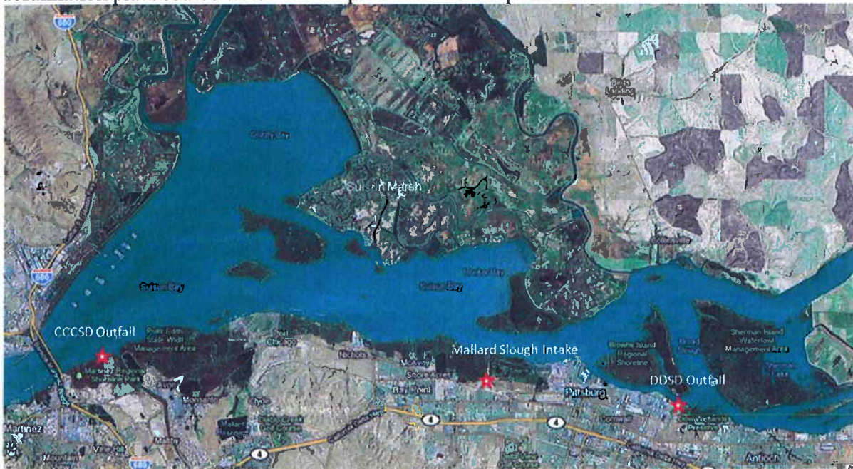
Figure 1 Map showing proposed desalination plant at Mallard Slough Intake and two possible brine disposal sites, Central Contra Costa Sanitary District (CCCSD) and Delta Diablo Sanitation District (DDSD).
